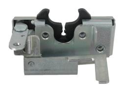
This two rotor latch is designed for medium to heavy-duty applications for off highway entrance doors where push button handle actuation is desired. It features an integrated linkage that allows for direct push button actuation and direct inside release and provides for ease of mounting and applications.
